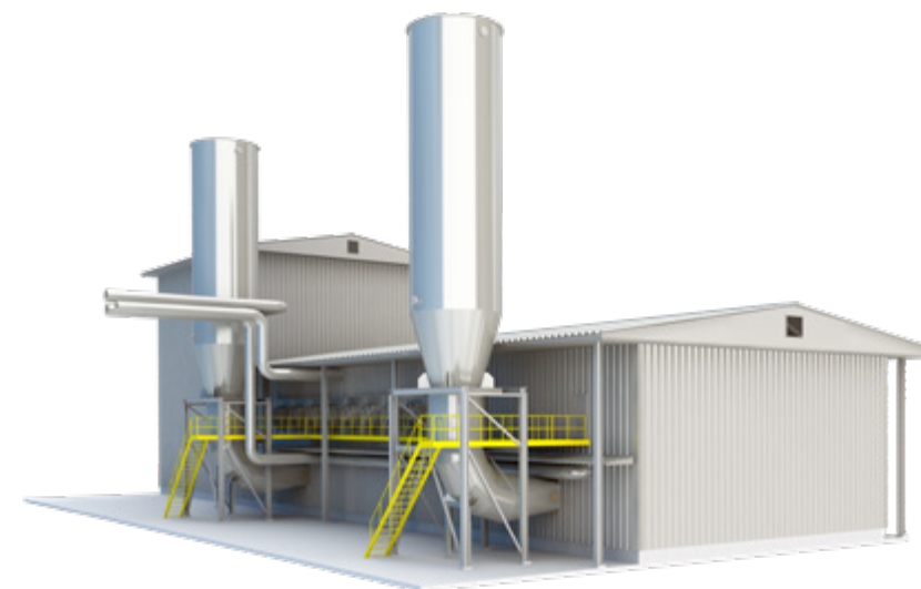
This belt dryer has been protected using a spark detection system that controls a dry sprinkler system which has been installed above the perforated belt.
