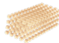
Chopped wood sawed into cubes of 1 cm Fire area 5.4 m 2 (58.1 ft 2 )
